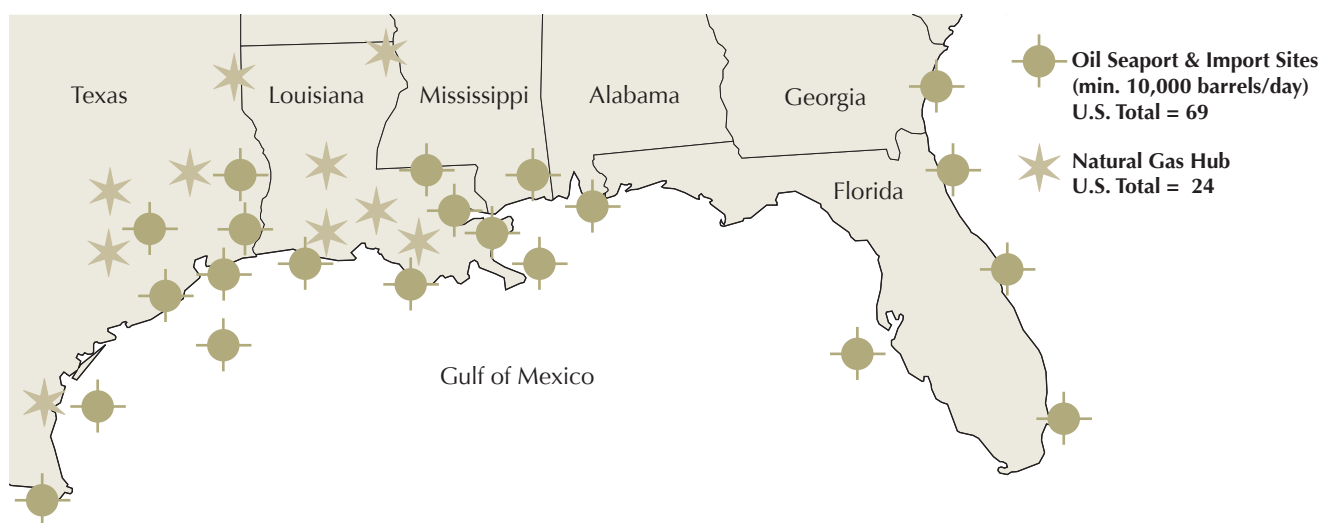
FIGURE 14: Oil and gas industry infrastructure along the Gulf Coast.
